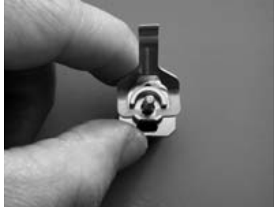
Fig. 9 – Correct Lever Orientation
