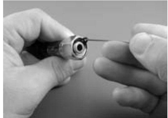
Fig. 2 – Removal of LP Hose O-ring
