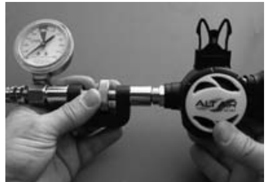
Fig. 13 – Inline Adjustment Tool w/ IP Gauge
