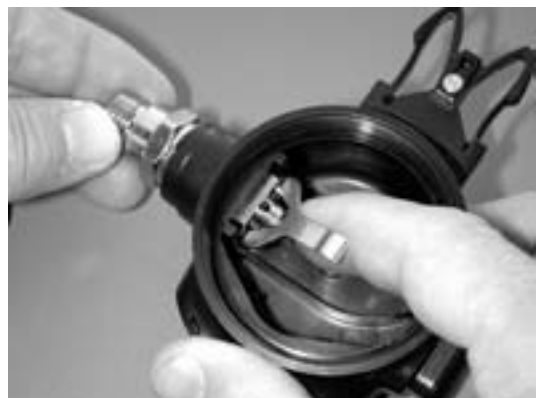
Fig. 11 – Installation of Inlet Fitting
