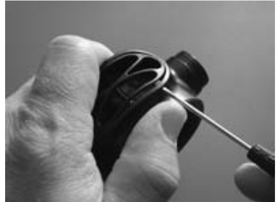
Fig. 6 – Exhaust Grill Removal
