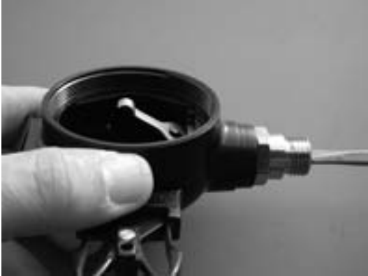
Fig. 12 – Preliminary Setting of Orifice
