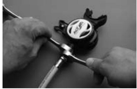
Fig. 1 – Removal of LP Hose
