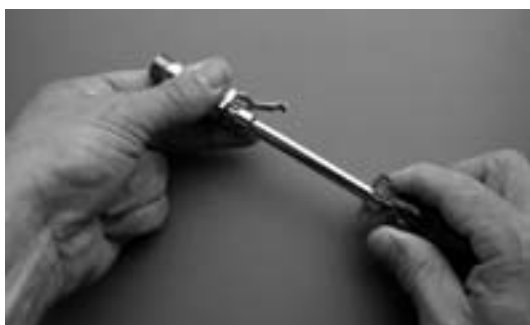
Fig. 5 – Disassembly of Valve Mechanism
