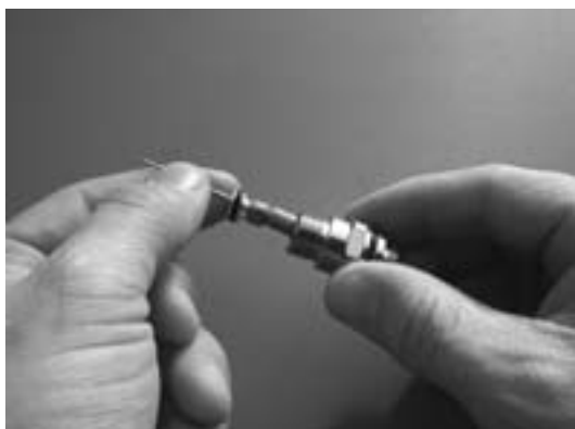
Fig. 3 – Removal of Adjustable Orifice
